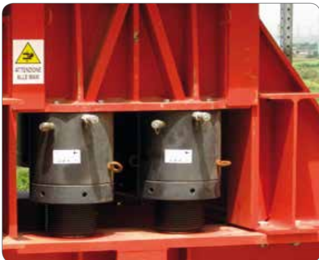
CRI 200/100 GS TA double-acting cylinders with safety ring for lifting structures.
