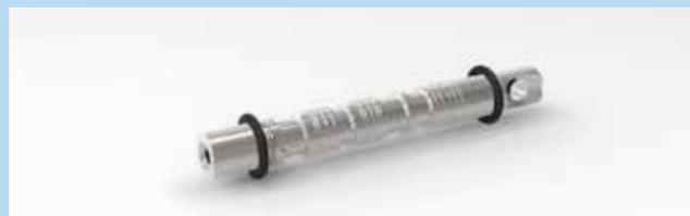
Regenerative spool in position 2. The regenerative circuit allows the cylinder double-acting to increase its speed, in one way only, adding to the pump flow the oil returning from the rod chamber of the cylinder. Special machining on the body is required.
