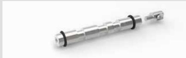
Double-acting spool regenerative in position 3, for valves with right inlet. The regenerative circuit allows the cylinder to increase its speed, in one way only, adding to the pump flow the oil returning from the rod chamber of the cylinder. To be combined only with spool controls 42 or 43. Special machining on the body is required.
