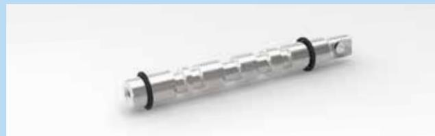
Same features as spool A with the addition of a fourth floating position. The floating position allows a cylinder to float or a motor to wheel free when the spool is in position 3. To be combined only with spool controls 12, 13. Special machining on the body is required.
