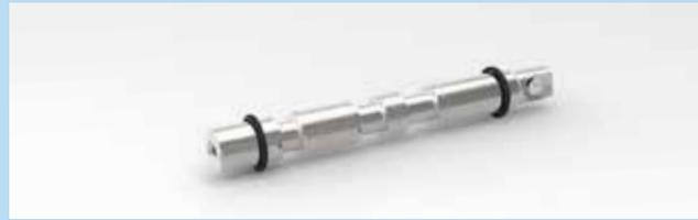
Spool with regenerative circuit in position 3. The regenerative circuit allows the cylinder to increase its speed, in one way only, adding to the pump flow the oil returning from the rod chamber of the cylinder. To be combined only with spool controls 14, 26, 42 or 43. Special machining on the body is required.
