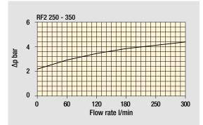
The curves are plotted using mineral oil with density of 0.86 kg/dm<sup>3</sup> in compliance with ISO 3968. Ap varies proportionally with density.
