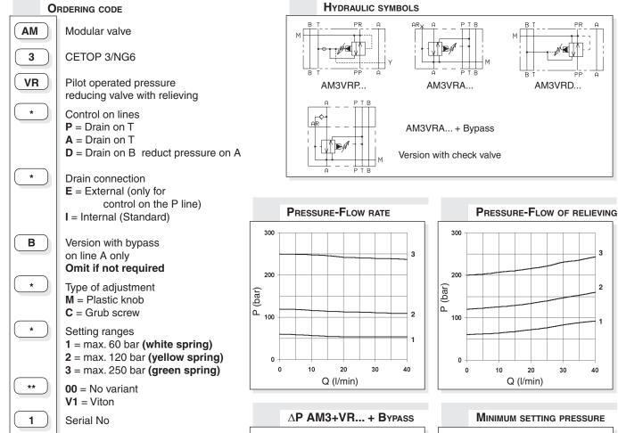
To changes valves AM3VRP... from internal to external drainage it is necessary: - screw out the plug on the "Y" port
