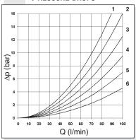
The diagram at the side show the pressure drop curves for spools during normal usage. The fluid used is a mineral oil with a viscosity of 46 mm²/s at 40°C; the tests have been carried out at a fluid temperature of 40°C.
