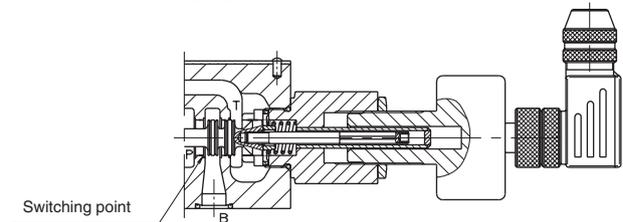
**NB:** connecting the output to Pin 4 or Pin 2 the type of contact, normally closed or open, can be chosen.
