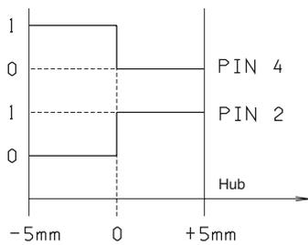
0 = Voltage Pin 2 and Pin 4 < 1,8 V
