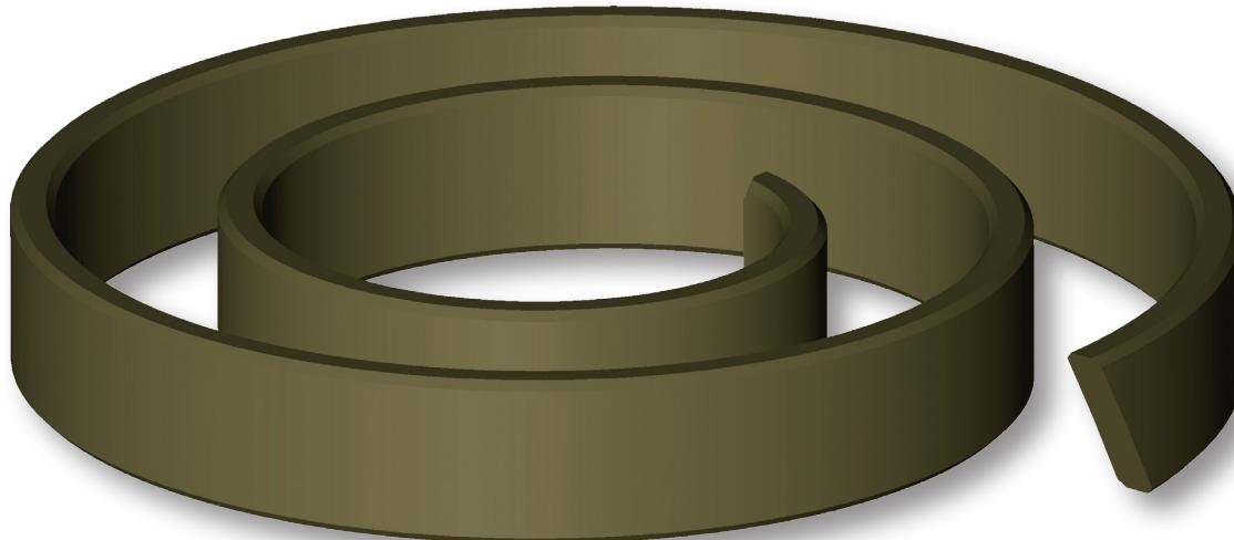
The Aston Seals MRB type guide rings have been developed to substitute traditional bronze guides in hydraulic cylinders. They guide the rod or the piston and prevent metallic contact with the cylinder when radial forces act perpendicular to the direction of movement.
