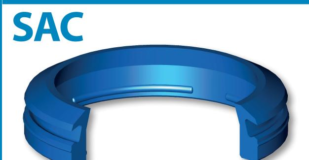
The function of the Aston Seals SAC wiper ring is to prevent introduction of dust, dirt and foreign matter into the system, to protect the guiding parts and to extend the service life of the axial moving rod seals.
