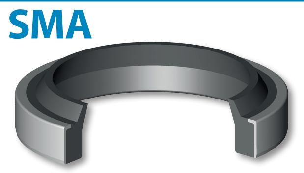
The function of the Aston Seals SMA wiper ring is to prevent introduction of dust, dirt and foreign matter into the system. This is achieved by a special wiper lip which produces a very effective cleaning action, prevents the development of scores, protects the guiding parts and extends the service life of the axial moving rod seals.
