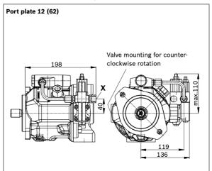
A10V(S)O Series 31 | Axial piston variable pump 24 Dimensions, size 28
