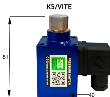
"K5" adjustable pressure switches activate a microswitch once preset value is reached. The pressure is set by rotating a graduated knob or, for the economical version, by a setscrew located on top of the unit. Both systems are supplied with a device permits locking the desired set pressure. Mechanical stops protect both the spring and the microswitch from over pressurization.
